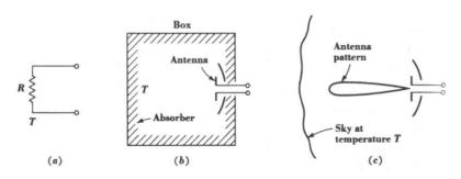
Fig. 3-24. (a) Resistor at temperature T; (b) antenna in an absorbing box at temperature T; and (c) antenna observing sky of temperature T. The same noise power is available at the terminals in all three cases.
