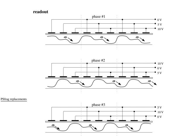
During the exposure phase, electrons promoted to the conduction band in the semiconductor are collected in a potential well under each pixel. The well is created by holding the central electrode in each pixel at a more positive potential than its neighbours.
